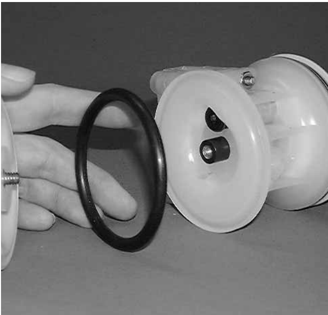
Step 9. Figure 9 Pull off Teflon®/PTFE diaphragm and O-ring. ( Figure 9 ) Twist off remaining diaphragm in counter-clockwise direction. Inspection of diaphragms and O-rings is now possible.
